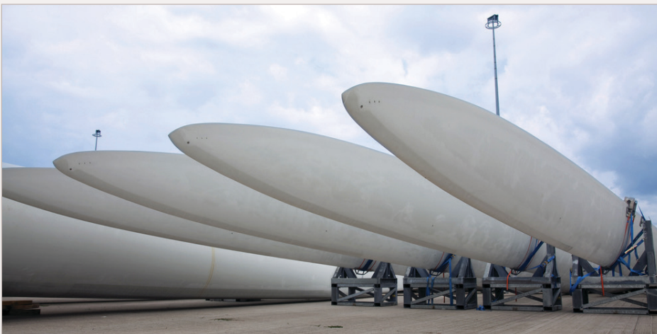
Composite wind turbine blades awaiting installation
